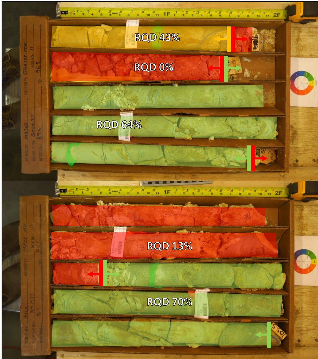
Figure 13-10: GM19-37 Core Trays (89.5 to 105.5 ft.) – High Variability in Geotechnical Conditions
