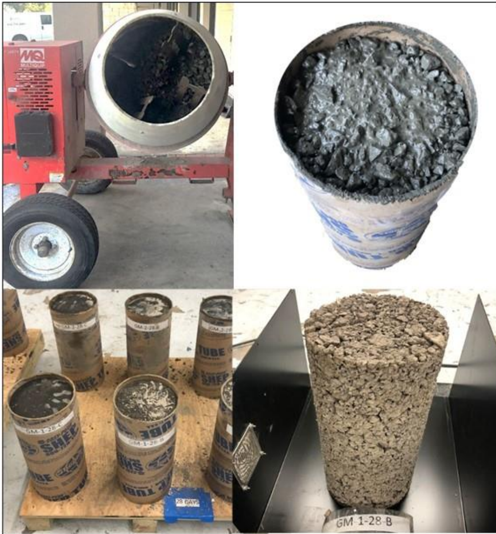
Figure 13-29: Mixing, Casting and Curing Process
