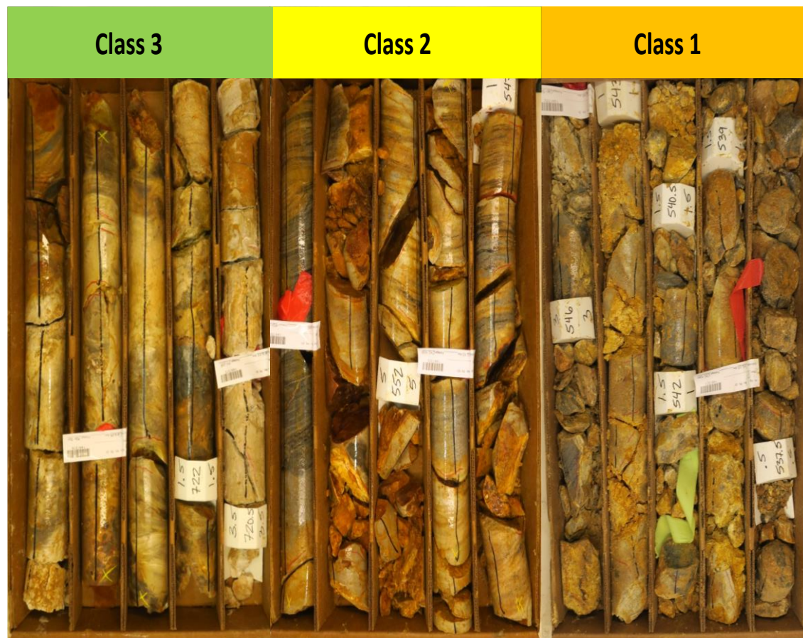
Figure 13-9: Examples of Three Geotechnical Rock Classes
